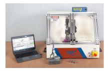
The <u>CNC Test Device</u> (CNCTD) is designed to screen and train for CNC setup operators with production responsibilities. The device provides a means of quantitatively screening for CNC setup operator positions, for use in evaluating job applicants and as a grading device for training purposes.
