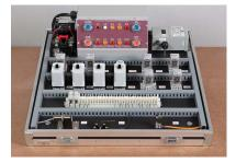
Our <u>Electrical Skills Test Device</u> (ESTD) is designed to screen and train for industrial electricians and electro-mechanical production positions. The device provides a means of quantitatively screening candidates for industrial electrician positions, for use in evaluating job applicants and as a grading device for training purposes.
